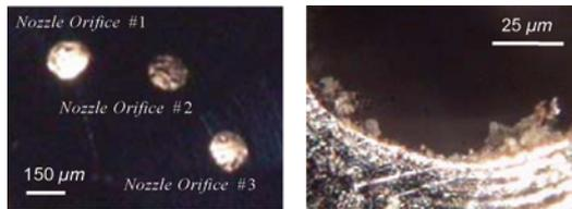
(a) Nozzle Orifice #1, #2, and #3 (b) Detailed inlet image of Nozzle Orifice #3
